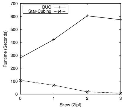
Figure 17: Star-Cubing vs. BUC w.r.t. Skew, where  $\mathcal{T} = 1M$ ,  $\mathcal{D} = 10$ ,  $\mathcal{C} = 10$ ,  $\mathcal{M} = 100$
