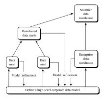
Figure 4.2: A recommended approach for data warehouse development.
