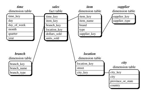
Figure 4.7: Snowflake schema of a data warehouse for sales.
