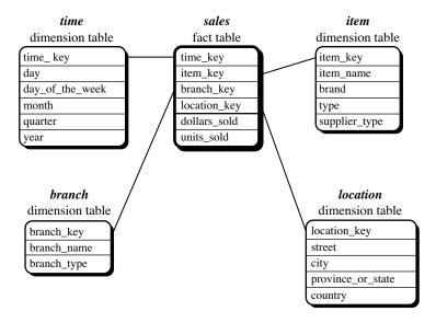
Figure 4.6: Star schema of a data warehouse for sales.
