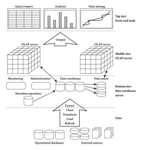
Figure 4.1: A three-tier data warehousing architecture.
