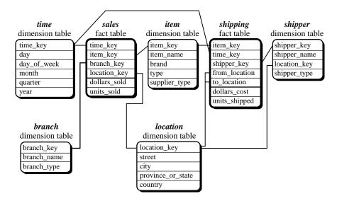
Figure 4.8: Fact constellation schema of a data warehouse for sales and shipping.
