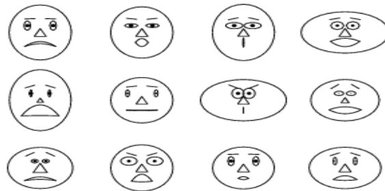
Figure 2.17: Chernoff faces. Each face represents an n -dimensional data point ( n \leq 18 ).
